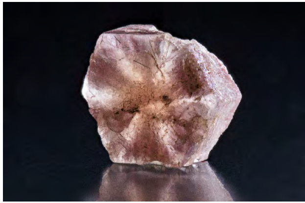
Figure 7. As viewed through the pinacoid face, strong oblique fiber-optic lighting illuminates the six-legged trapiche structure emanating from the c-axis of this doubly terminated 2.33 ct pezzottaite crystal. Photo by Kevin Schumacher.
