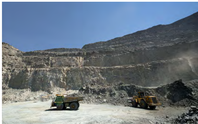
Figure 13. A 50-ton dump truck and front-end loader remove the kimberlite ore after blasting at the bottom of the Main diamond pipe. Photo by Robert Weldon/GIA; courtesy of Letšeng Diamonds.
