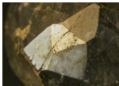
Figure 16. Diffused reflected light exposed spotty luster on the surface of one of the tested stones, indicating the presence of a coating. Field of view 2.17 mm.
