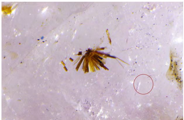
Figure 10. Using diffused transmitted and oblique fiber-optic illumination, a golden-brown spray of needles is shown deep in the crystal, along with a bright blue crystal to its right. Their depth precluded analysis by Raman spectroscopy. Photomicrograph by Nathan Renfro; field of view 0.91 mm.
