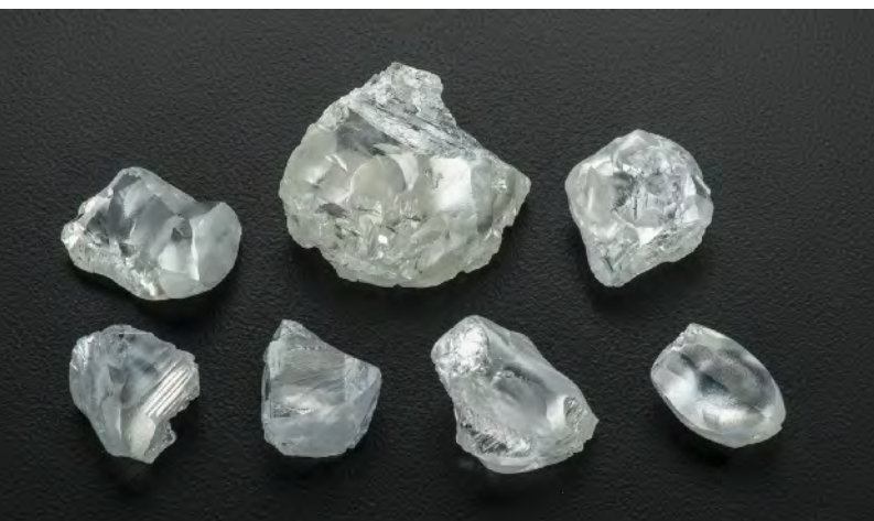
Figure 18. This group of type IIa rough diamonds ranges from almost 14 ct to 91.07 ct. Such diamonds make Letšeng a feasible mining proposition. Photo by Robert Weldon/GIA; courtesy of Gem Diamonds Ltd.
