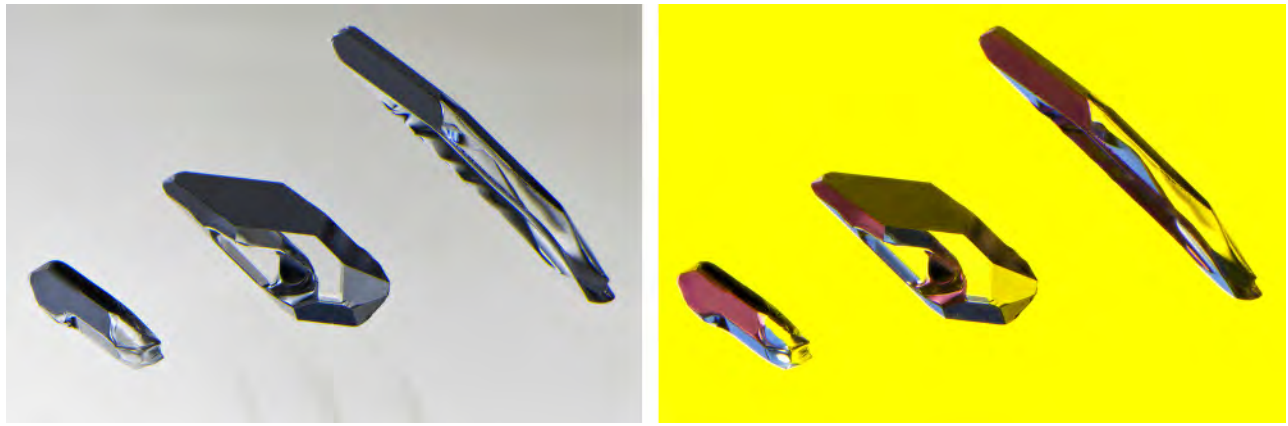
Figure 13. With modified Rheinberg illumination to impart contrasting color on some of the crystal faces, the negative crystals in the rock crystal quartz (left) prove to be crystallographically aligned (right). Photomicrographs by Nathan Renfro; field of view 7.34 mm.
