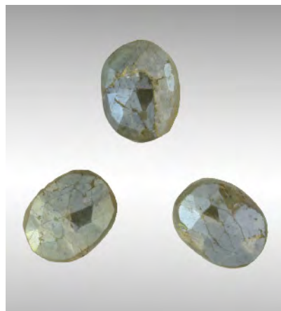
Figure 15. These three kornerupine beads (0.95–1.38 ct) were found to have a metallic coating.
