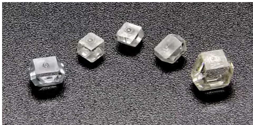
Figure 4. As-grown HPHT diamond single crystals produced using a simple Fe-based solvent with Al as a nitrogen getter. The sample on the far right is the largest, weighing 1.40 ct. Photo courtesy of New Diamond Technology.
