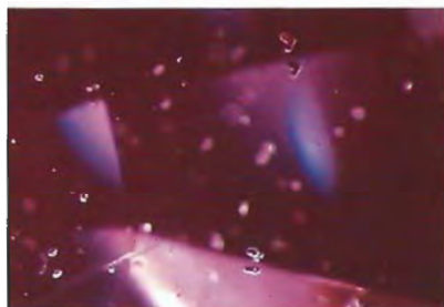
Figure 1. The transparent rounded crystals seen in this 3-ct flux-grown synthetic alexandrite are very unusual for this material. Magnified 45 \times .
