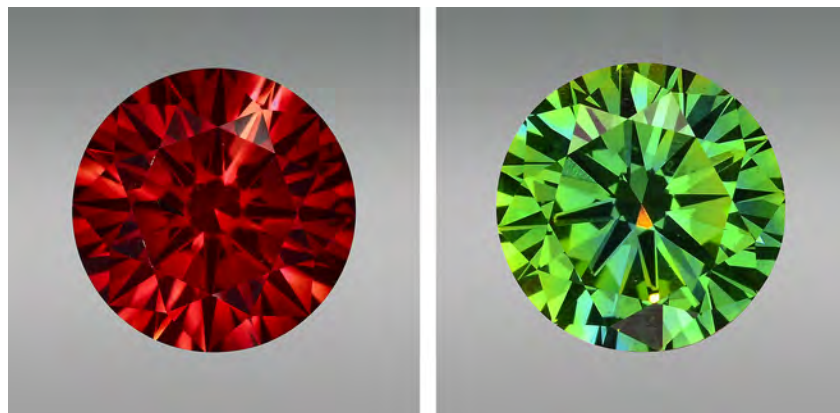
Figure 24. These two treated synthetic diamonds, a 0.57 ct Fancy red and a 0.50 ct Fancy Vivid yellowish green, show strikingly vibrant colors rarely found in natural-color diamonds.
