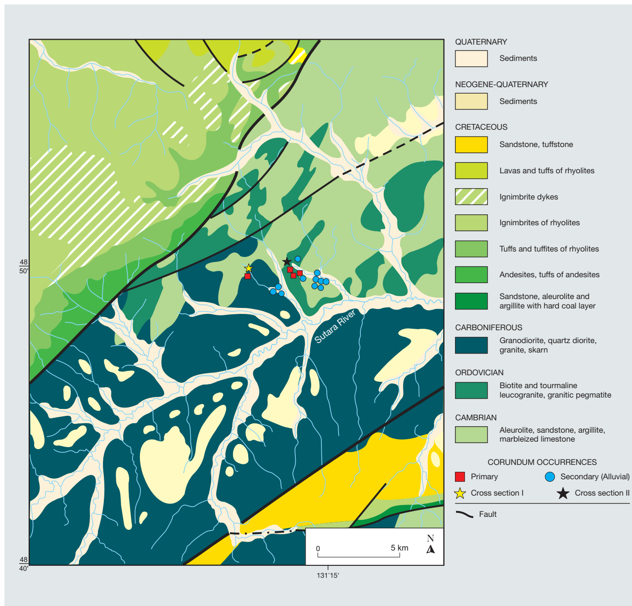
Figure 4. This simplified geologic map shows the primary and secondary (alluvial) sapphire occurrences discovered in the basin of the Sutara River. The basement is composed of metamorphosed carbonate rocks, intruded by granite and pegmatite. Adapted from Vaskin (1999).
