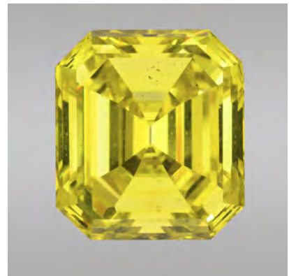
Figure 7. This 59.88 ct Fancy Vivid yellow diamond was treated through artificial irradiation and annealing.
