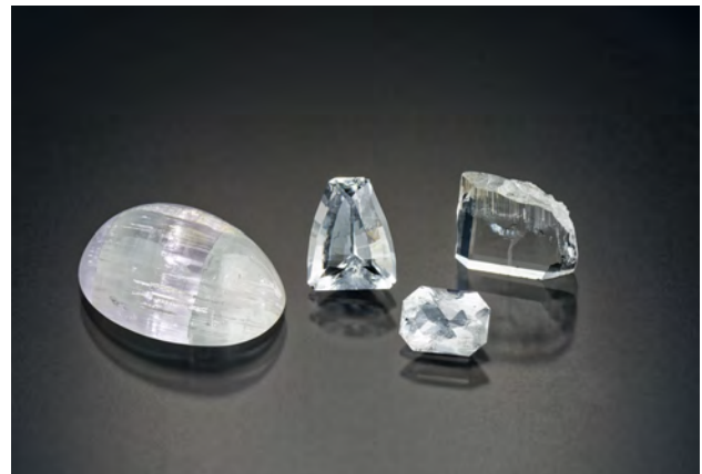
Figure 4. Left to right: a cat’s-eye beryllonite cabochon, two faceted transparent colorless samples, and a partially polished specimen with clean areas and growth tubes. The larger faceted stone in the center weighs 1.90 ct. The rough on the far right is the specimen from this study. Photo by Kevin Schumacher.
