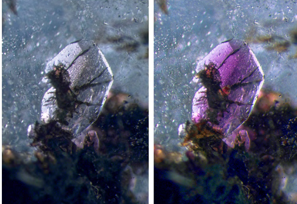
Figure 15. With plane-polarized light, the axinite inclusions in quartz show very distinct pleochroism. Both of these images were taken with the polarizer rotated at approximately 90 degrees from each other. Photomicrographs by John I. Koivula; field of view 9.0 mm.
