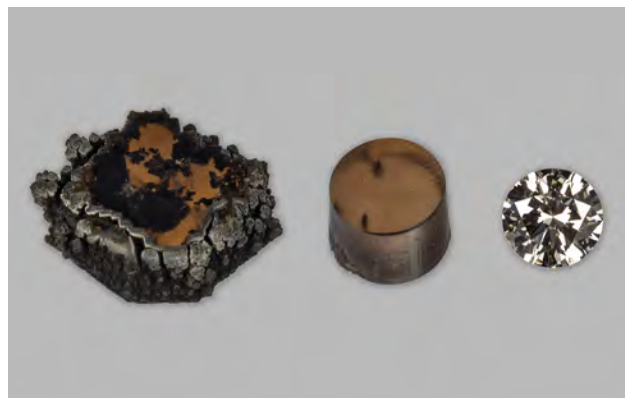
Figure 3. An as-grown 4.52 ct CVD-grown crystal with a graphitized outer edge and a brownish color (left), a CVD synthetic diamond crystal laser-cut to a 1.91 ct cylinder (center), and a 0.40 ct near-colorless, heat-treated CVD round brilliant (right). Note these are three separate samples at different post-growth stages and should not be interpreted as a progression of the same sample. Photo by C.D. Mengason.
