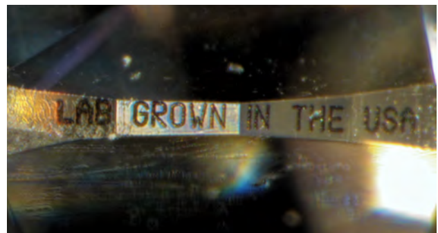
Figure 9. Most CVD manufacturers inscribe their products as laboratory-grown on the girdle, as in this photo. Similarly, all samples identified as synthetic diamonds leave GIA with an identifying inscription of “Laboratory Grown.” Photo by Sally Eaton-Magaña.
