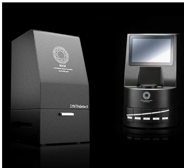
Figure 1. The De Beers Group instruments SYNTHdetect (left) and AMS2 (right) provide screening capability for melee-size diamonds as small as 0.3 points. Photo courtesy of Danny Bowler © De Beers Group.
