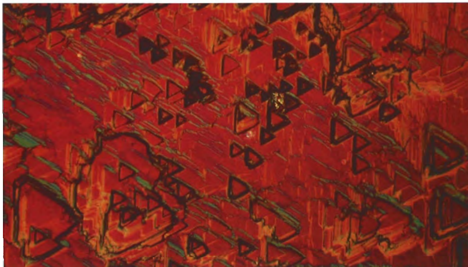
Figure 12. Natural spinel crystals like this one commonly have triangular etch features. Photomicrograph by John I. Koivula; magnified 80×
