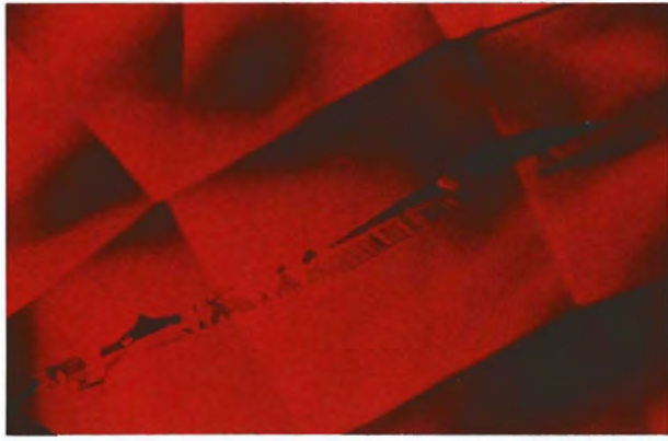
Figure 5. Dark reddish to orangy brown, jagged-edged flux inclusions (with gas bubbles), such as this 3-mm-long example, provide proof that the host stone is synthetic. Note how the inclusions taper to a point. Photomicrograph by John I. Koivula.
