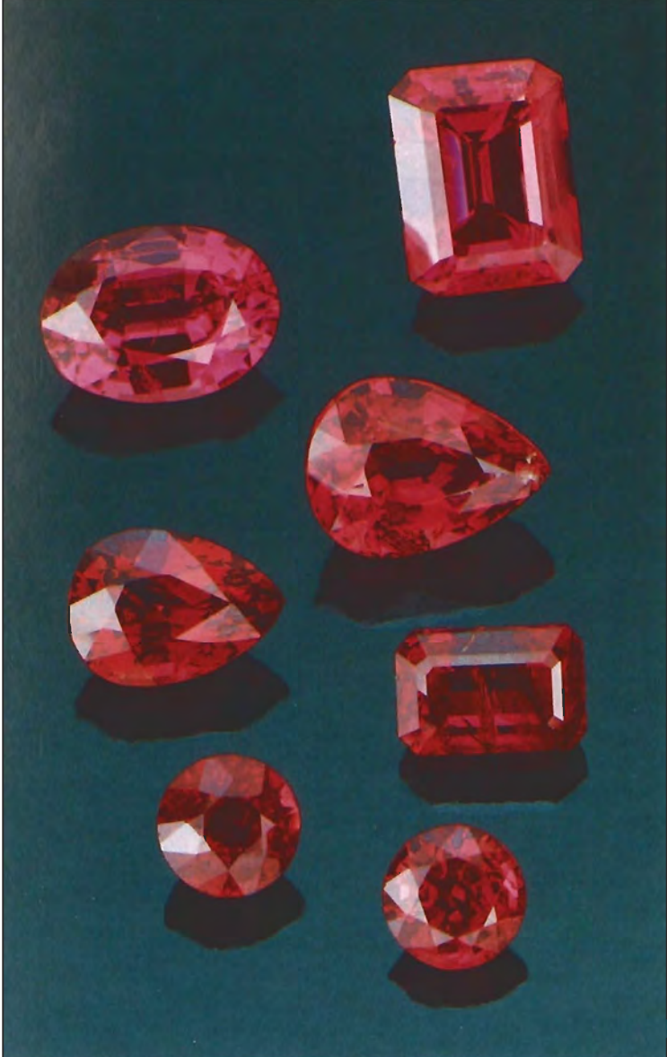
Figure 1. These faceted Russian flux-grown synthetic red spinels (the largest is 2.27 ct) are representative of those examined during this study. Photo © Tino Hammid and GIA.
