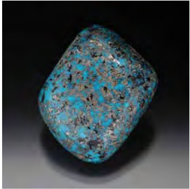
Figure 51. This 59.59 ct freeform turquoise cabochon contains numerous sulfide inclusions. The dark spots are Superglue-filled cavities. Courtesy of Jack Lowell; photo by Robert Weldon.
