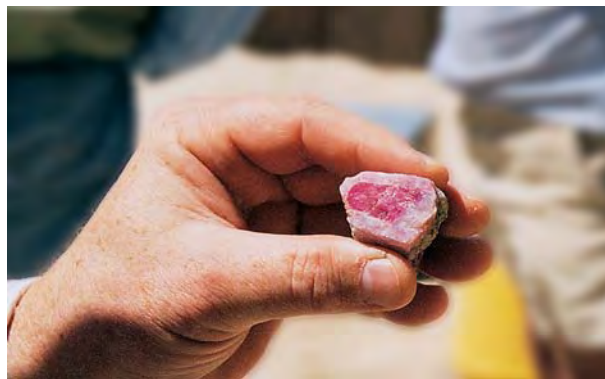
Figure 13. Strong color zoning is common in the rubies from the John Saul mine, as this basal section of a stone from the Kimbo pit illustrates. Photo © John L. Emmett.
