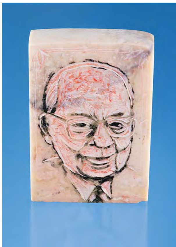
Figure 5. Raman spectra taken on this printing block "stone" carving of GIA Chairman Richard T. (Dick) Liddicoat, Jr. matched that of the mineral dickite. Photo by Maha Tannous.
