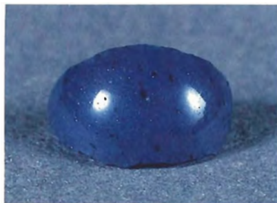
Figure 13. This quartzite bead (which measures approximately 8 mm) was dyed to imitate lapis lazuli.
