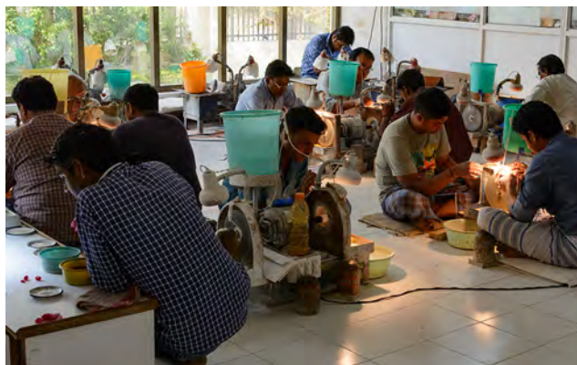
Figure 20. Sambhav's preformers and faceters are shown cutting morganite and fire opal. Photos by Andrew Lucas, courtesy of Sambhav Jewels.
