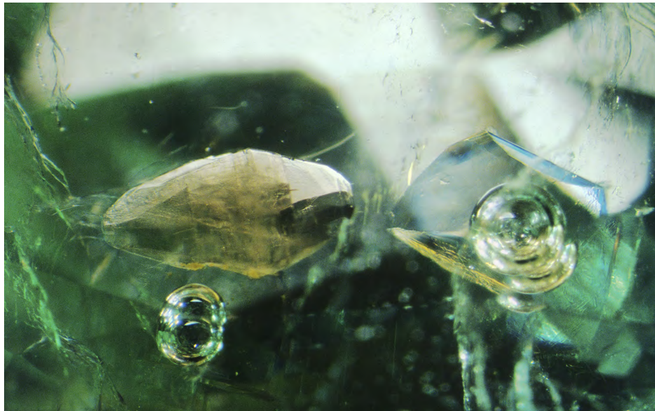
Figure 1. This emerald contains a brown crystal of the rare mineral parisite. There is also an oil-filled cavity showing a blue and orange flash effect, along with two large trapped gas bubbles. This inclusion suite verifies the natural origin of this emerald; it also confirms that the stone, which shows signs of clarity enhancement, is from Colombia. Photomicrograph by John I. Koivula; field of view 3 mm.
