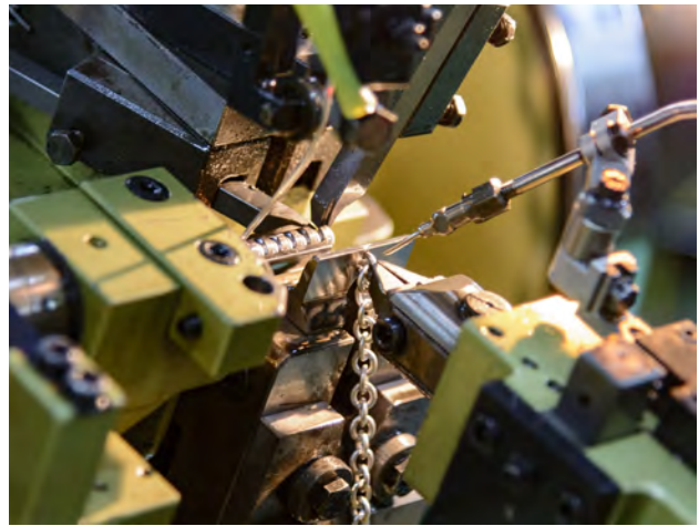
Figure 36. An assortment of chain-making machines in Derewala's factory are capable of creating numerous styles in silver and various gold karat alloys. Photo by Andrew Lucas, courtesy of Derewala.
