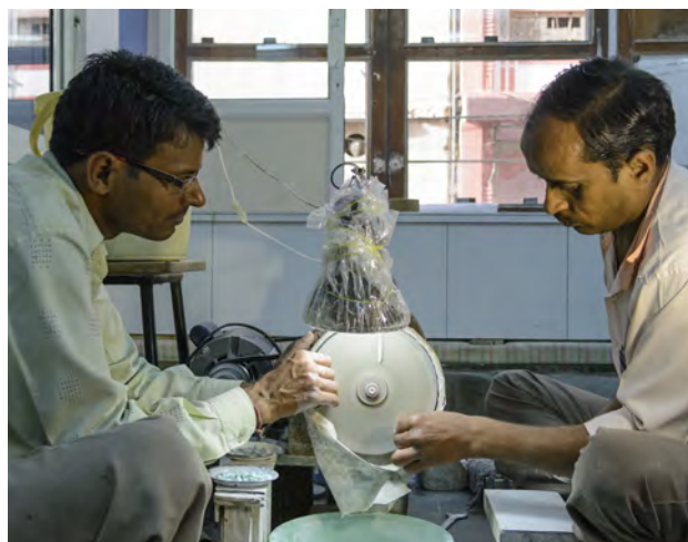
Figure 21. National Facets uses the cottage industry for cutting but prefers to preform for beads and cabochons in its own factory, as this is a critical stage for weight. Photo by Andrew Lucas, courtesy of National Facets.
