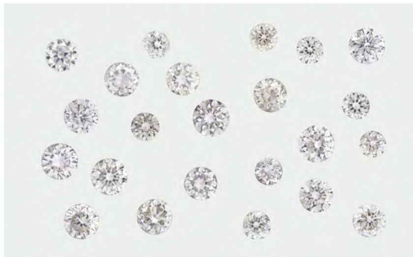
Figure 16. These 23 HPHT-grown synthetic diamond melee, ranging from 0.002 to 0.012 ct, were identified recently at GIA's Hong Kong lab.
