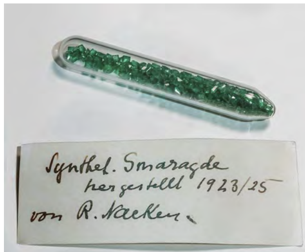
Figure 2. This glass vial containing 360 faceted and 10 rough synthetic emeralds was donated by Nacken in 1961 to Munich's Deutsches Museum. The diameter of the vial is approximately 10 mm. Photo courtesy of Deutsches Museum.
