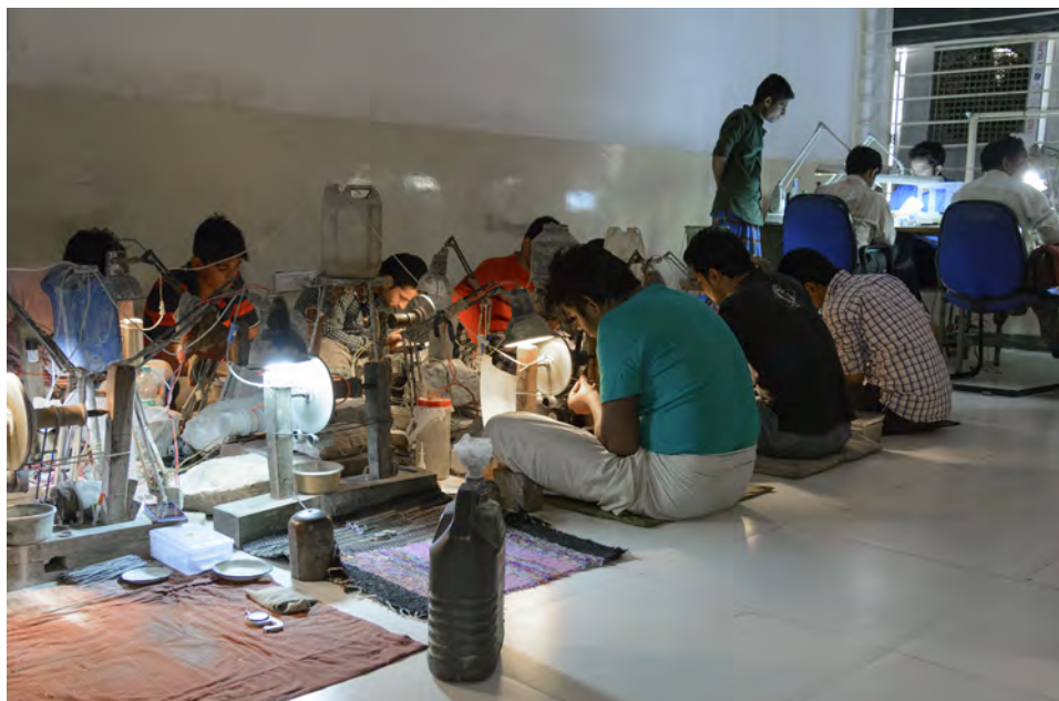
Figure 14. M&M Gems has a traditional Jaipur factory where preformers prefer to work sitting on the floor. Each preformer averages 400 stones a day. Photo by Andrew Lucas, courtesy of M&M Gems.
