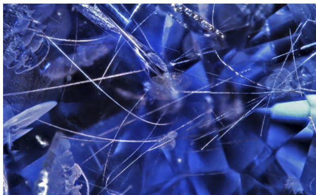
Figure 8. Curved linear features with healed fissures. The image was taken using a combination of dark-field and fiber-optic illumination. Photomicrograph by Victoria Raynaud/GIA; field of view 3.50 mm.
