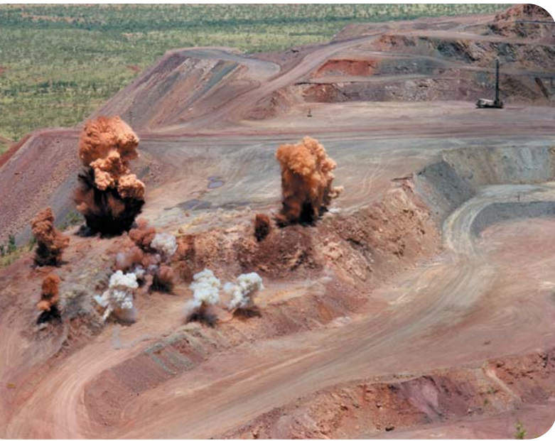
Figure 9. At Argyle, explosives are used to break up the lamproite ore and its overburden, so that it can be removed more easily.
