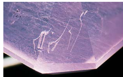
Figure 5. Elongated, thready gas bubbles in this color-change apatite proved its synthetic origin. Magnified 20 \times .
