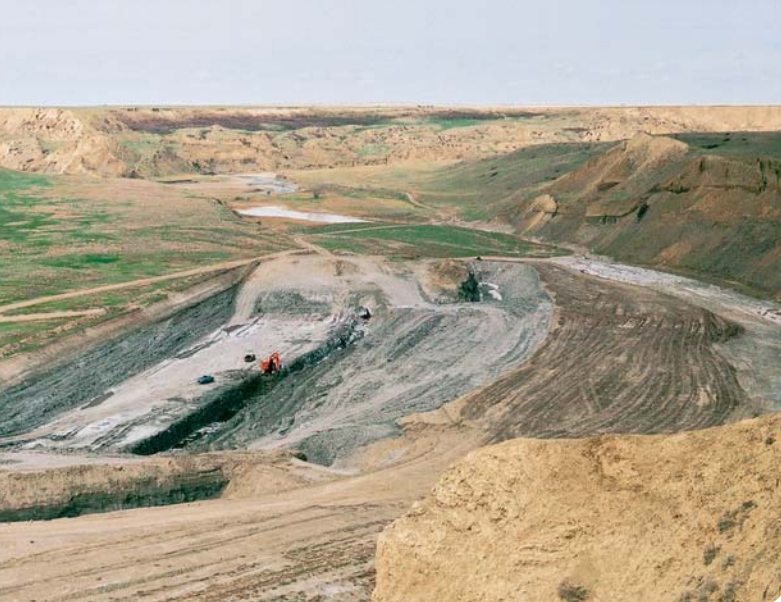
Figure 4. The open-pit Oxbow mine, located on the Blood Indian Reserve, currently is the main source of Ammolite. An orange-colored backhoe, sitting directly on the K Zone (see text), is barely visible in the center of the photograph. The St. Mary River (not visible) runs along the base of the cliff in the distance. Note on the left side of the pit that the lighter soil represents alluvial deposits, whereas the underlying gray stratum is the Bearpaw Formation. The cliff on the right caps the gray Bearpaw Formation with tan-colored glacial sediments. Photo taken looking north; courtesy of Korite International.
