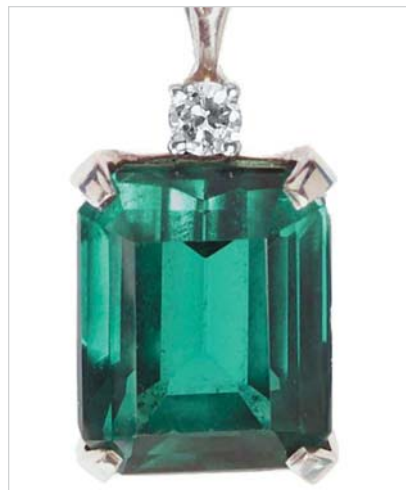
Figure 6. The transparent green imitation emerald (10.00 × 8.00 × 6.35 mm) in this pendant was identified as an assemblage consisting of a colorless beryl crown of undetermined origin and a green glass pavilion joined by a colorless layer of cement.
