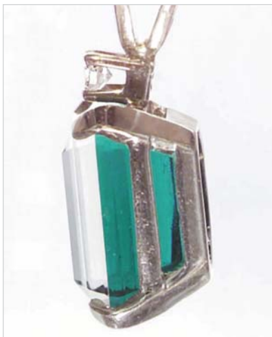
Figure 7. Immersion in water eliminates the optical illusion of this assembled emerald imitation, and the true colors of the crown and pavilion can be seen.
