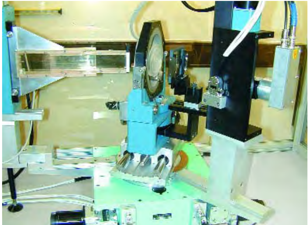
Figure 15. In the X-ray topographic apparatus used in this study, the diamond is held in the circular goniometer array (20 cm in diameter) in the top-center of the photo. The X-ray beam enters from the left, and the film is positioned on the right side of the goniometer. Photo by Nikolaus Herres.
