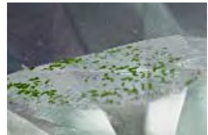
Figure 5. The green radiation stains in this faint pink diamond generally have well-defined boundaries. Length of this image is about 4 mm.
