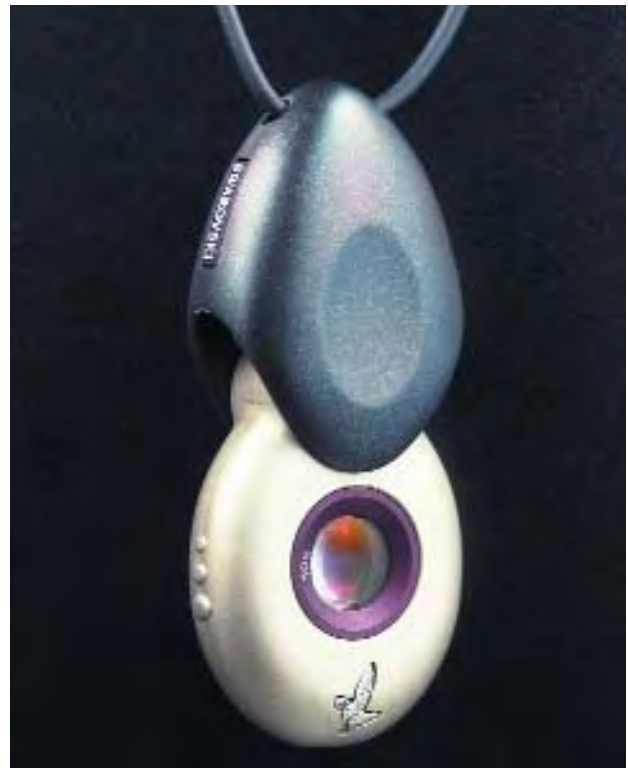
Figure 30. This newly developed 10 \times loupe from Swarovski Optik has several innovative features, including an ergonomic design and a much lighter lens. Photo by Elizabeth Schrader.
