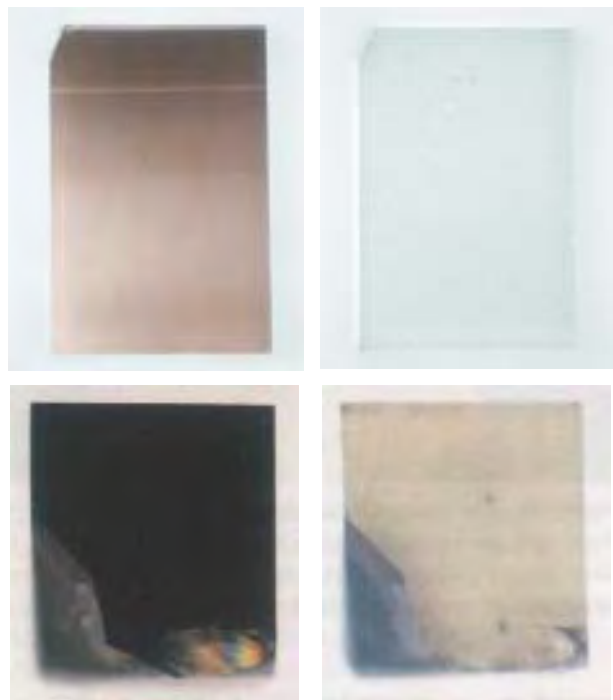
Figure 17. These photographs illustrate how two N-doped CVD synthetic diamond samples that started as brown (top left, 3.06 \times 2.06 \times 0.86 \text{ mm}^3 ) and black (bottom left, 1.52 \times 1.34 \times 0.94 \text{ mm}^3 ) responded to HPHT treatment (right). Photos by A. Taylor.
