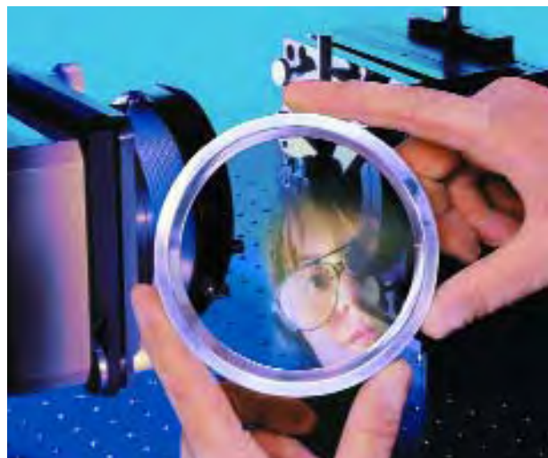
Figure 3. The polycrystalline CVD synthetic diamond optical window shown here was manufactured by Element Six and has a thickness of 0.68 mm. Polycrystalline material has a range of technical uses, but it is extremely difficult to polish into anything resembling a traditional gemstone. Photo courtesy of Element Six Ltd.
