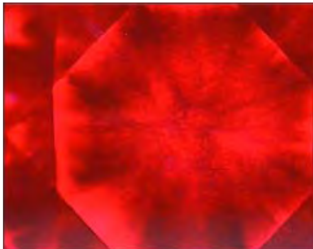
Figure 25. There are rare instances in which DiamondView images of a natural type IIa diamond will show orange luminescence throughout. In such cases, we have observed underlying networks of dislocations of a kind that we have not seen for CVD synthetic diamond. (Imaged area: 3.6 mm × 2.7 mm.) Photo by S. Lawson.
