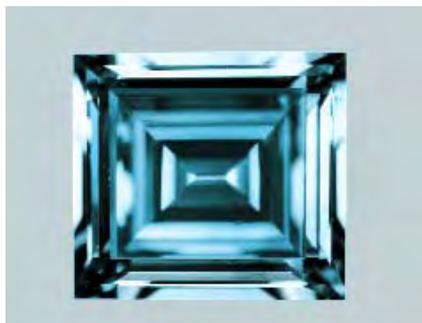
Figure 5. This 1.03 ct Fancy Deep blue square-cut CVD synthetic ( VS_2 clarity, type IIb) was grown with diborane added to the process gases. Photo by M. Crowder.
