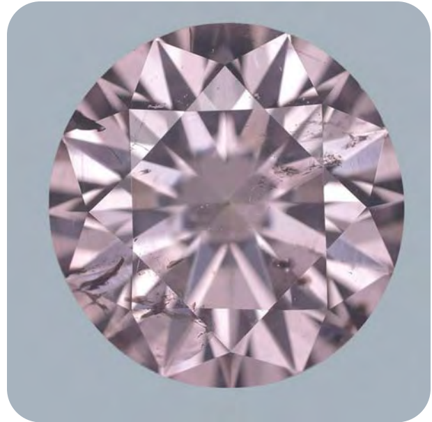
Figure 1. This 0.85 ct purple-pink diamond was examined at the DTC Research Centre to investigate the claim that it had been HPHT treated. Careful analysis and observation revealed that the color of the diamond was due to a topical coating that had been applied to the pavilion of the stone. Photo by Chris Kelly.
