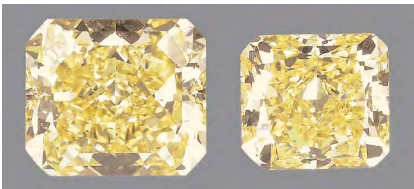
Figure 3. This 4.33 ct rectangular modified brilliant cut (left) proved to be a type IIa HPHT-treated diamond. In contrast to many other HPHT-treated type IIa diamonds, it shows a pure yellow color that is surprisingly similar to the 1.21 ct untreated type Ia cape stone on the right, which was also color graded as Fancy yellow.
