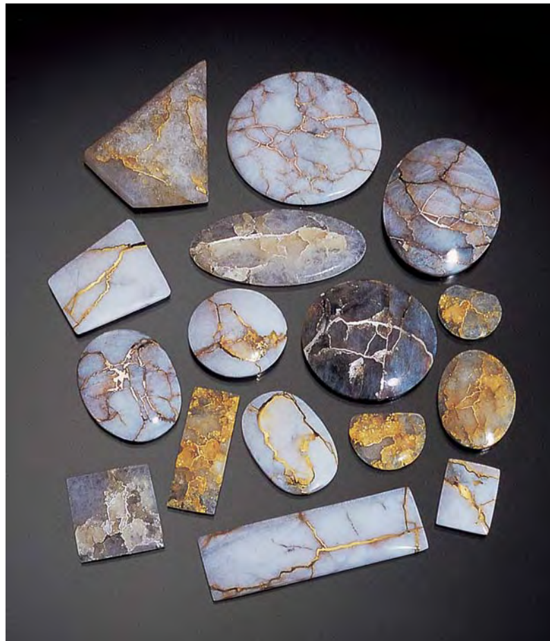
Figure 19. A new process is being used to introduce gold and silver into smoky, milky, and colorless quartz for jewelry use. The elongate piece on the bottom measures 52 x 30 mm. Courtesy of Eureka Gems LLC; photo © Jeff Scovil.
