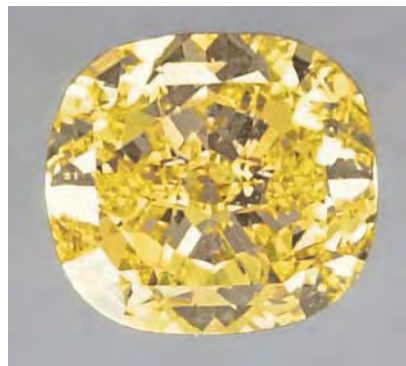
Figure 5. This natural-color 1.03 ct cape diamond showed localized H3 absorption, a feature typically associated with treated-color yellow diamonds.
