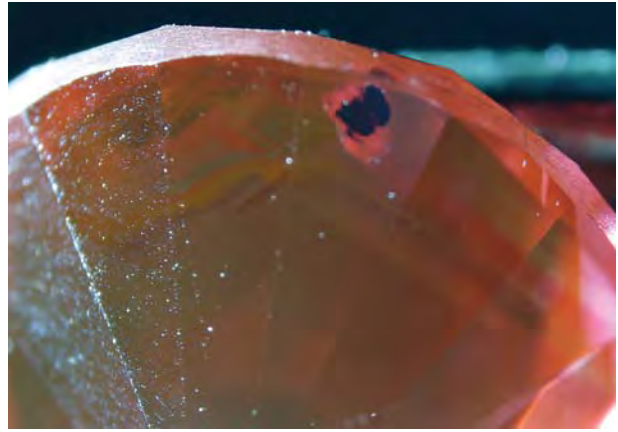
Figure 15. Strikingly, when exposed to a strong light source, several of the samples exhibited all three luminescence colors—green, orange-red, and yellow—producing a combination of colors unlike any the authors had seen previously in a natural-color diamond. Photomicrograph by C. P. Smith; magnified 27 \times .
