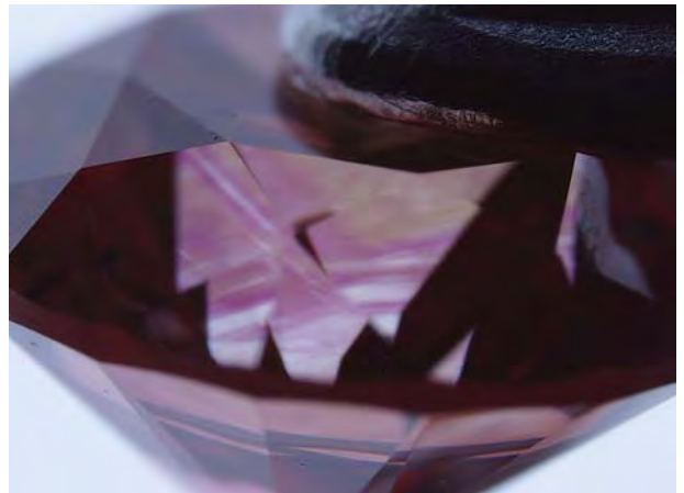
Figure 12. A few diamonds contained distinct pink-to-red zones in some areas, with brown and near-colorless zones in others. Photomicrograph by C. P. Smith; magnified 28×.
