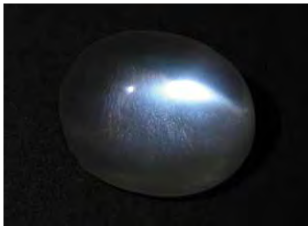
Figure 29. This 19.40 ct cabochon appears to show strong adularescence, but it proved to be a doublet imitating a high-quality moonstone. Photo by T. Hainschwang.
