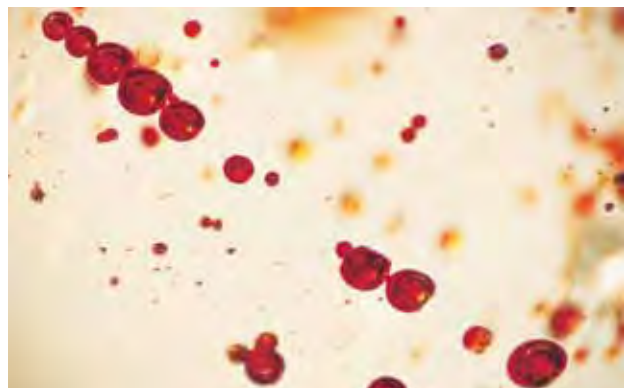
Figure 17. Strongly resembling a trail of blood, this row of brownish red fluid droplets was discovered in a polished specimen of copal resin from Colombia. Similar fluid inclusions in the sample contained movable gas bubbles. Photomicrograph by J. I. Koivula for microWorld of Gems ; magnified 15 \times .
