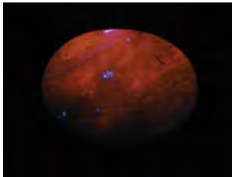
Figure 5. This attractive blue, 14.71 ct cabochon (sample no. FN-7692), reportedly from Mogok, appears to be a combination of massive haiüyne and sodalite. Note the strong zoned orange fluorescence to long-wave UV (right); the chalky blue spots correspond to the white areas seen in normal lighting. Photos by C. Grobon (left) and T. Hainschwang (right).
