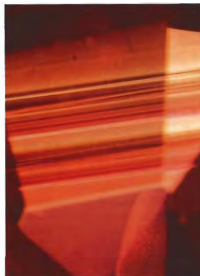
Figure 16. These straight, parallel, near-colorless and orangy red bands are not commonly seen in flux-grown synthetic rubies. Magnified 25×.
