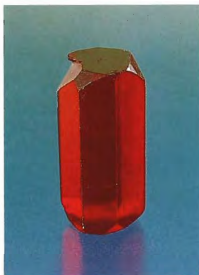
Figure 15. Although this vaguely resembles a red beryl crystal, it is actually a flame-fusion synthetic ruby. The piece measures 23.09 × 11.83 × 10.22 mm
