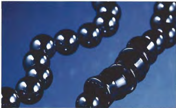
Figure 17. These 8-mm silicon beads (left) are being marketed as a "lighter" alternative to hematite (right). Photo by Maha Smith.
