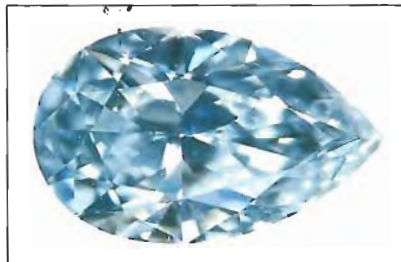
Figure 3. Routine testing of this 1.07-ct fancy gray-blue diamond revealed that it had unusually high electrical conductivity.
