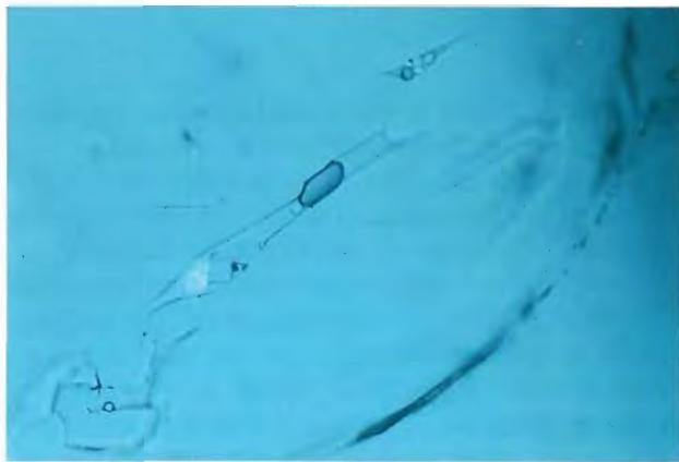
Figure 13. Multiphase fluid inclusions are common in Afghan emeralds. The larger inclusion here contains four isotropic and four anisotropic daughter minerals, brine (L), CO 2 -liquid (CL) and vapor (V). The inclined cubic habit of the largest isotropic phase is suggestive of halite (Ih). The lower refractive index isotropic mineral may be sylvite (Is). The identity of the other isotropic daughters (I) is unknown. The large rhombic daughter is probably a carbonate (Ac). The identity of the three smaller anisotropic minerals (A) is unknown. The CO 2 liquid forms a barely visible crescent between the vapor bubble and brine. The smaller inclusion contains two isotropic and two anisotropic daughter minerals in addition to brine and vapor. The length of the large inclusion is 200 μm. Photomicrograph by Robert R. Seal II; magnified 200×.
