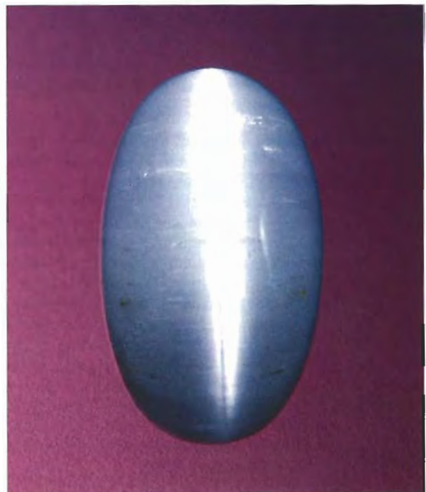
Figure 4. The chatoyancy in this 8.49-ct beryllonite (15.70 × 9.45 × 6.60 mm) is an unusual phenomenon for this material. Photo by Maha Smith.
