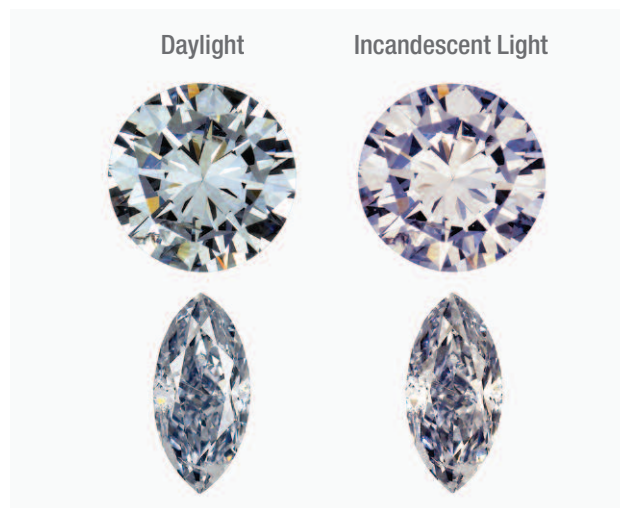
Figure 7. This 0.13 ct Fancy Light gray-blue diamond (top) and 0.33 ct Fancy grayish blue diamond (bottom) are colored by hydrogen defects and show a different color appearance with different light sources. Color grading occurs under daylight conditions (left), whereas incandescent lighting produces a more violet color (right).
