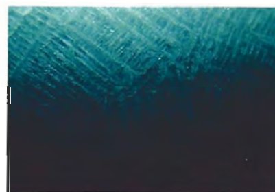
Figure 2. At 20x magnification, the cabochon shown in figure 1 revealed a dendritic pattern typical of man-made devitrified glass. Oblique illumination.
