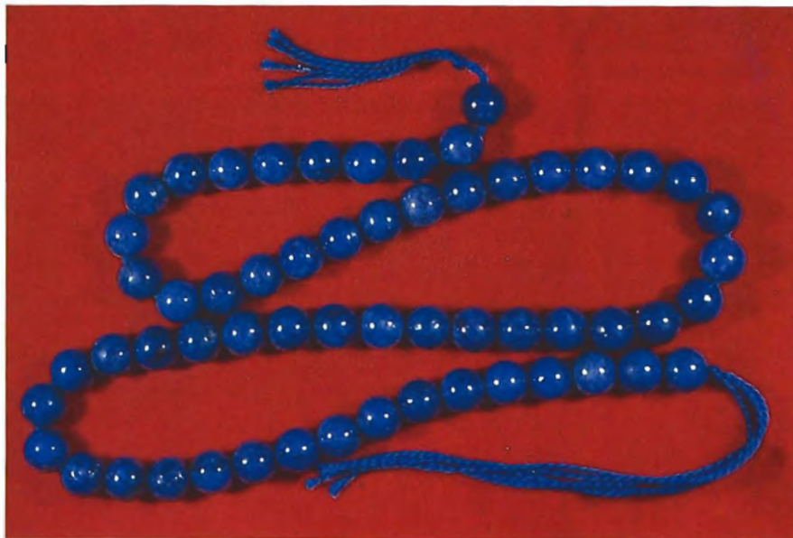
Figure 4. These 7-mm lapis lazuli beads were heavily dyed and then coated with paraffin.
