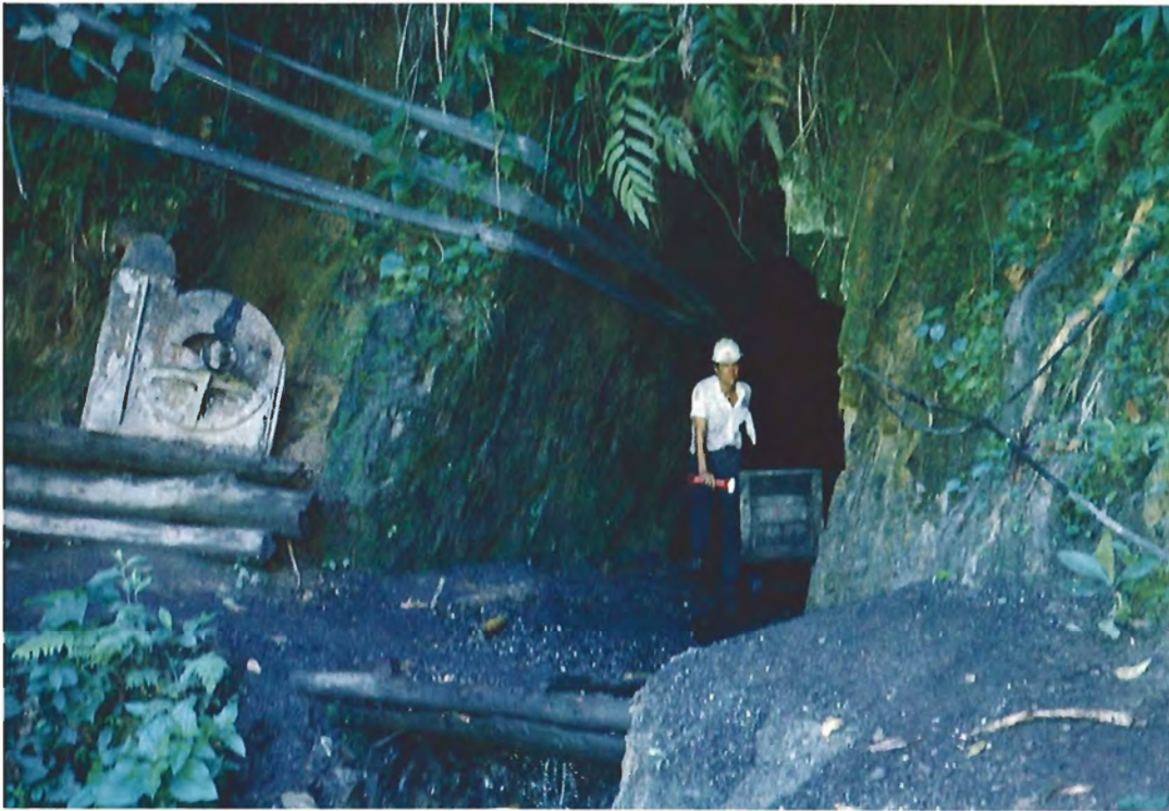
Figure 5. Below Coscuez, the Túnel la Tabla penetrates 600 m into the mountain as the miners follow the emerald-bearing calcite veins. Note the plastic tubes used to deliver air into the tunnel. Until recently, tunneling was the principal method of mining at Coscuez.
