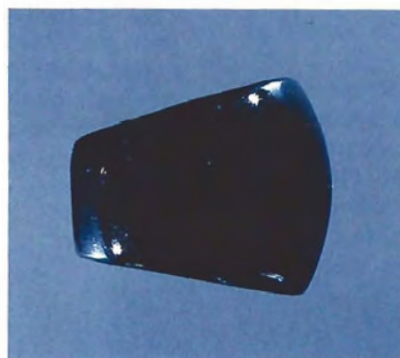
Figure 1. This 2.89-ct black free-form cabochon, represented as dyed black chalcedony, was found to be cobalt-bearing devitrified glass.
