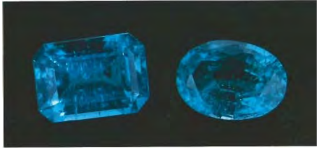
Figure 21. These beryl triplets (0.89 and 1.20 ct) are convincing imitations of the distinctive greenish blue tourmaline from Paraíba, Brazil. Photo by Maha DeMaggio.
