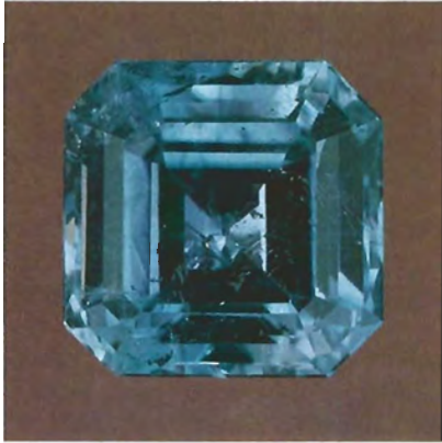
Figure 11. This unusual 1.85-ct greenish blue euclase was found to be colored by chromium.
