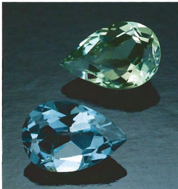
Figure 6. Ocean-green topaz sample 12 (top) showed no color change when exposed to combined fluorescent and incandescent (indoor) lighting. Sample 13 (bottom) changed from green to blue within a day of exposure to direct sunlight. Photo © GIA and Tino Hammid.
