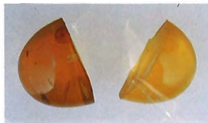
Figure 4. Originally, both portions of this 25 × 18 mm cabochon were dark. The section on the right faded when it was exposed to the light from a 14-watt Tensor lamp for approximately 170 hours at close range.
