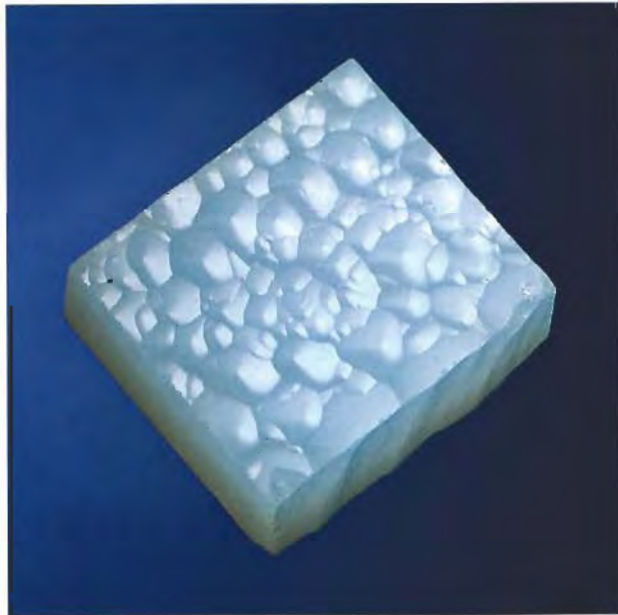
Figure 23. This 63.69-ct specimen (23.17 × 20.93 × 10.83 mm) is the first translucent synthetic quartz examined by the editors. Courtesy of Bob Lewis, Gems Galore ; photo © GIA and Tino Hammid.
