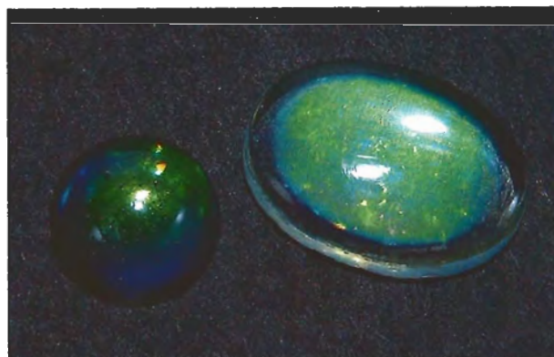
Figure 18. The 8.67-ct opal simulant on the right employs glass and a holographic image to imitate play-of-color; the 1.68-ct piece on the left consists of an interference-imaged film and an acrylic cabochon. Courtesy of Manning International; photo by Maha DeMaggio.
