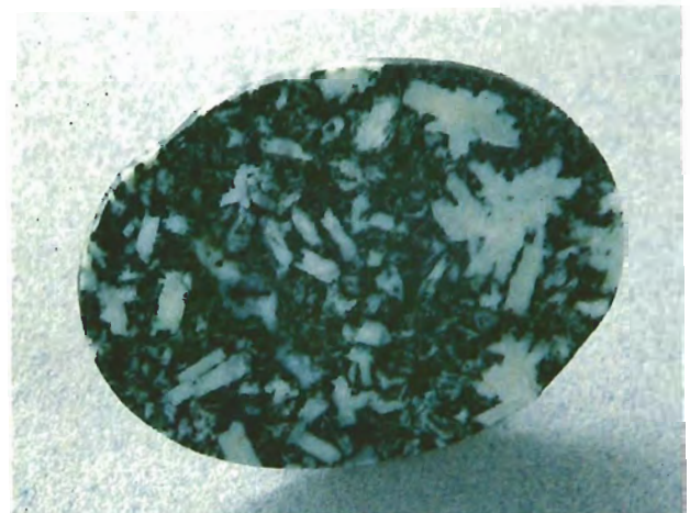
Figure 11. Marketed as "Flower Rock," this ornamental material (37.90 ct, 25.01 × 34.44 × 6.15 mm) is a dark porphyry with light-colored feldspar phenocrysts. Courtesy of West Coast Semi-Precious Stone; photo by Maha DeMaggio.
