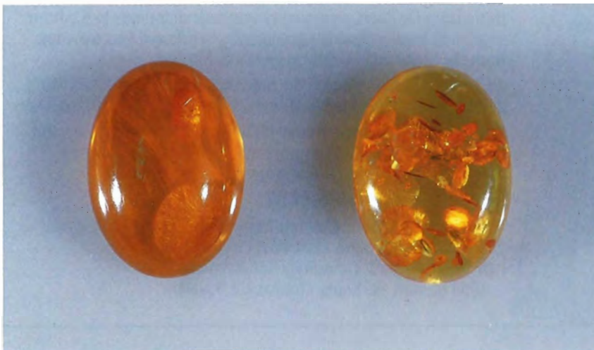
Figure 1. These two clarified amber cabochons (each about 25 × 18 mm, 10.50 ct) were from the same lot and, originally, both the same color. The paler specimen (right) had faded over time while displayed in a brightly lit case.
