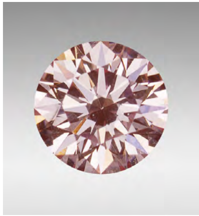
Figure 12. This 0.26 ct pink synthetic diamond contains the first H4 defect GIA has observed in a CVD synthetic diamond.
