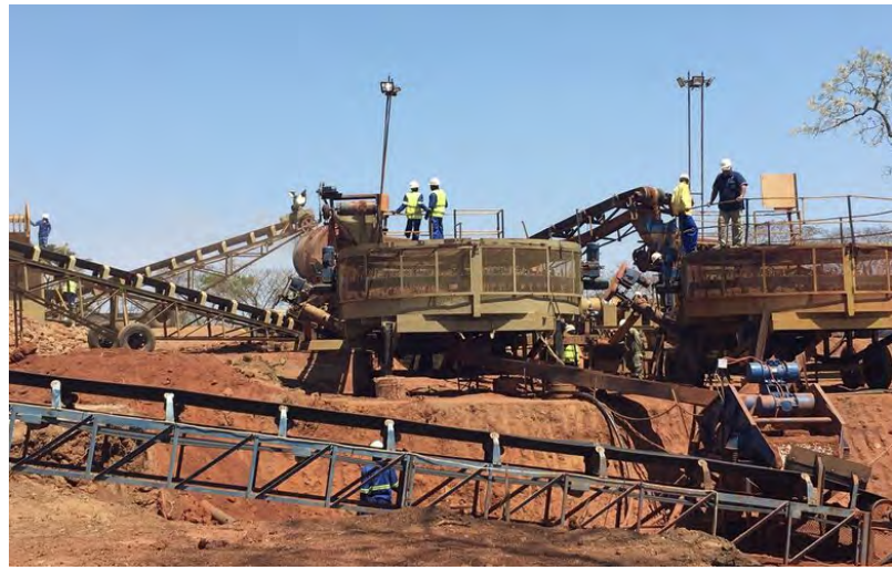
Figure 16. The washing process used by Mustang Resources is different from most jigs used for colored stone mining. Photo courtesy of Mustang Resources.
