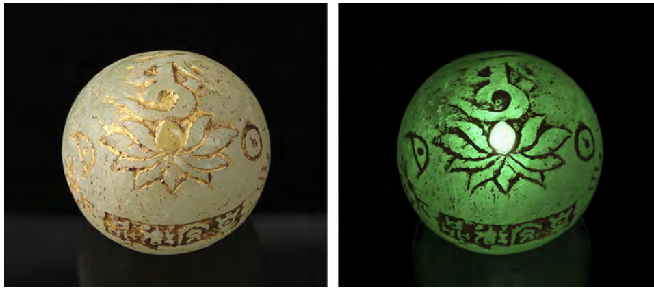
Figure 57. The calcite object (left, in daylight-equivalent light) showing a moderate green overall phosphorescence after short-wave UV exposure (right). The object emits a very strong whitish phosphorescence from one area, as seen in the center of the right image. Photos by Lai Tai-An Gem Lab.
