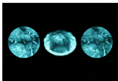
Figure 16. These DiamondView fluorescence and phosphorescence images of a 0.081 ct sample show growth patterns characteristic of HPHT synthetic diamond.
