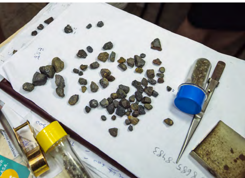
Figure 20. The polycrystalline form of diamond known as carbonado was first found in Bahia in about 1841. During the late 19th century, this very hard material was of great economic importance for industrial use. Shown here is a privately held collection of samples in the town of Lençóis. Photo by Robert Weldon/GIA.
