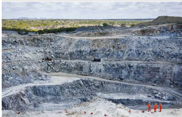
Figure B-1. A recent view of the open pit at the Lipari diamond mine near Nordestina in Bahia (left). The Braúna 3 kimberlite pipe lies beneath serpentinized soil and sedimentary rocks. Also shown is the processing plant on-site where kimberlite ore is broken down to recover the diamonds (right). Photos by Andrew C. Johnson, courtesy of Lipari Mineração Ltda.
