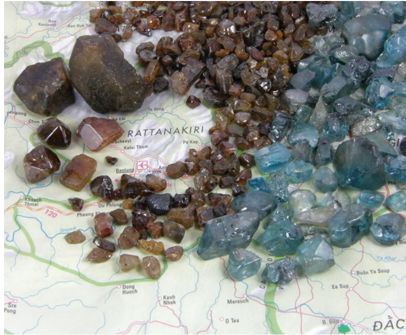
Figure 23. These rough zircons were recovered from Ratanakiri Province, Cambodia. The blue rough (up to 7 g) was produced by heating brown stones such as those on the left (up to 24 g). Photo by Prasit Prachagool.
