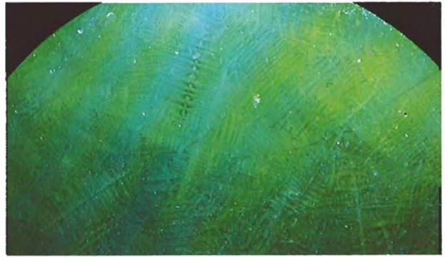
Figure 9. "Metajade" glass often shows a fern-leaf pattern under magnification. Here, magnified 5 \times .
