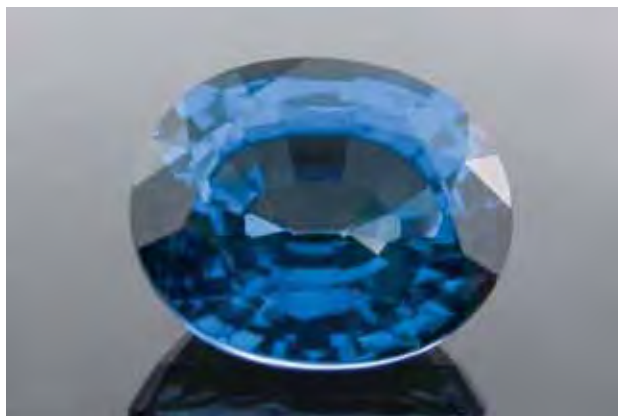
Figure 45. This 5.85 ct blue oval mixed cut was identified as a flame-fusion synthetic sapphire treated by a diffusion process. Photo by C. Golecha.
