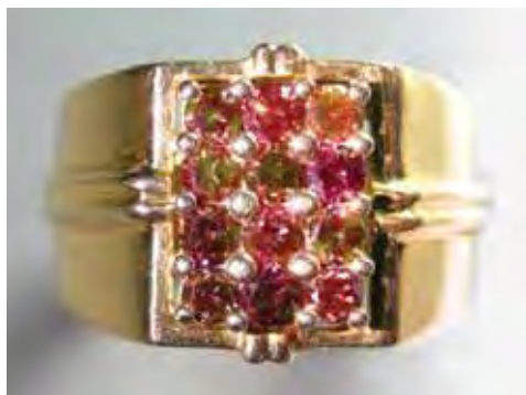
Figure 32. The round brilliants in this ring (average 2.8 mm diameter) proved to be treated-color pink synthetic diamonds. With strong fiber-optic illumination (right), nine of them showed unevenly distributed green luminescence. Photos by S. Singbamroong, © Dubai Gemstone Laboratory.
