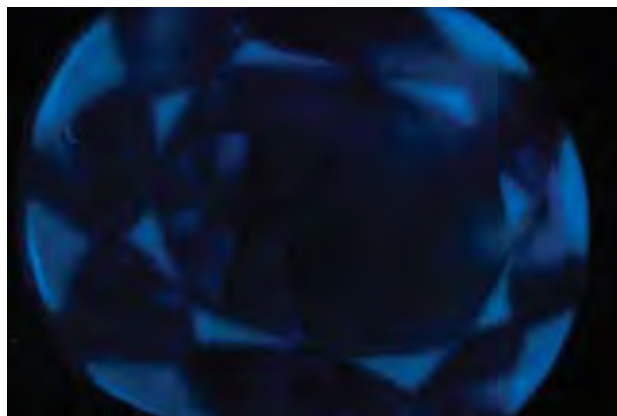
Figure 46. When exposed to short-wave UV radiation, the diffusion-treated synthetic sapphire in figure 45 showed an unusual pattern of symmetrical chalky blue fluorescence: The star and upper girdle facets fluoresced chalky blue, while the table, kite, and pavilion facets were inert. Photo by C. Golecha.
