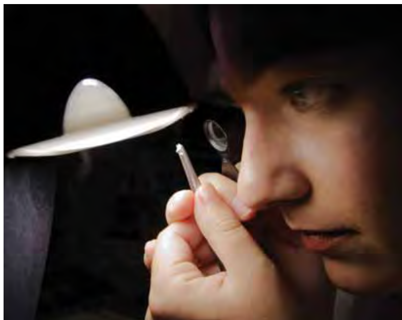
Figure 7. A consistent observation methodology is critical to assess the effect of graining on clarity. The final determination is made with a loupe as the diamond is held under the microscope's overhead light source—approximately 2–3 inches (5–8 cm) below the light source and in an area between the front edge of the lamp casing to approximately 2 inches beyond that edge. A black background is placed behind the light and the stone to keep the visual field clear and create a dark field for viewing. Photo by Valerie Power.
