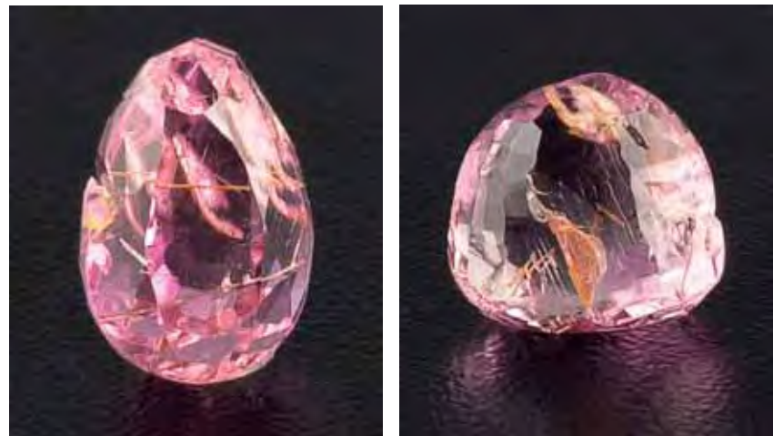
Figure 11. This 3.90 ct poudretteite (9.45 × 10.04 × 6.58 mm) is the first ever submitted to the GIA lab (face-up, left). Eye-visible orange-yellow epigenetic staining is present in both “fingerprints” and needle-like growth/etch tubes (pavilion up, right).
