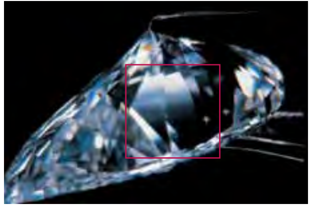
Figure 11. One type of whitish graining that usually affects the clarity grade is banding (i.e., alternating cottony or sheen-like lines or bands with dark areas between, as in figures 1 and 2). Whitish graining that has a more amorphous appearance, as illustrated here, and does not diminish transparency when observed through a range of motion, would not affect the clarity grade. Photomicrograph by Vincent Cracco; magnified 12 \times .
