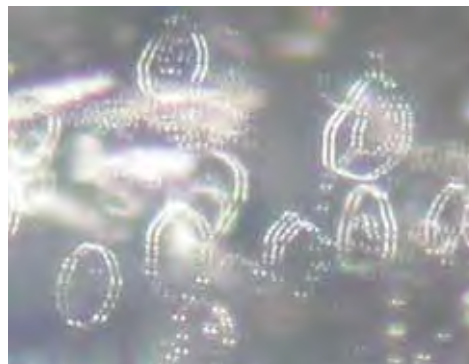
Figure 44. The ring-like inclusions in the sapphire (left) are indicative of high-temperature heat treatment (in this case by a traditional surface-diffusion process). At higher magnification, the circular inclusions were seen to be composed of fine particles. Photomicrographs by G. Choudhary; magnified 25× (left) and 70× (right).
