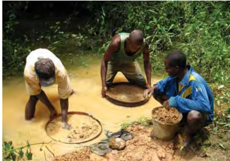
Figure 3. Most diamond mining in Sierra Leone exploits alluvial deposits. Here, diamond-bearing gravels are screened by independent miners. Photo by R. Taylor.
