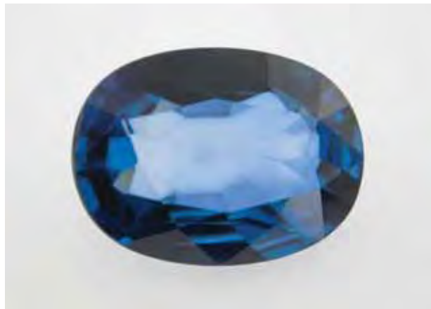
Figure 41. This 6.64 ct blue sapphire showing uneven patchy coloration owes its color to diffusion treatment. Photo by G. Choudhary.
