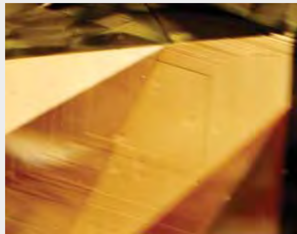
Figure A-4. Transparent internal graining that follows a diamond's octahedral growth sector typically has a square or rectangular outline. This type of graining typically fades in and out of view as the diamond is moved; it is not common for such graining to impact the clarity grade. Photomicrograph by W. Wang, magnified 40×.
