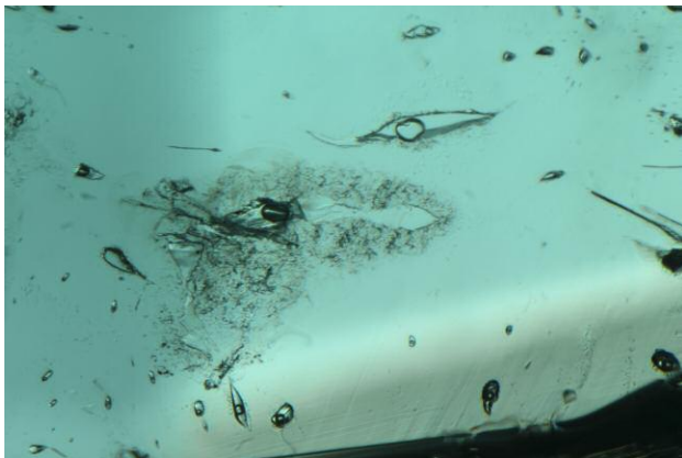
Figure 48. Irregular fluid inclusions with granular fringes in a Russian emerald. Photomicrograph by Aaron Palke; field of view 1.26 mm.
