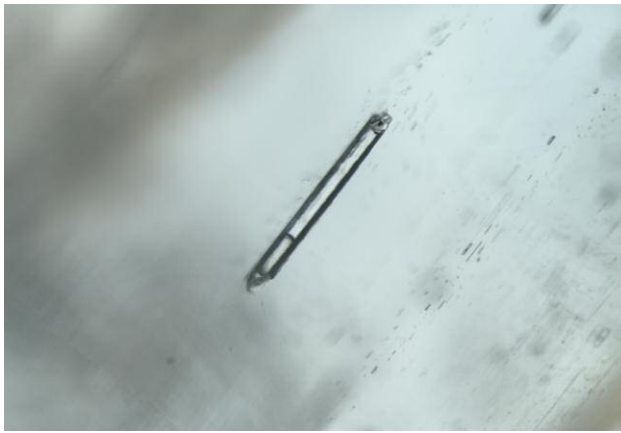
Figure 44. Elongate fluid inclusion with a small solid inclusion at the end in a Russian emerald. Photomicrograph by Suwasan Wongchacree; field of view 1.20 mm.
