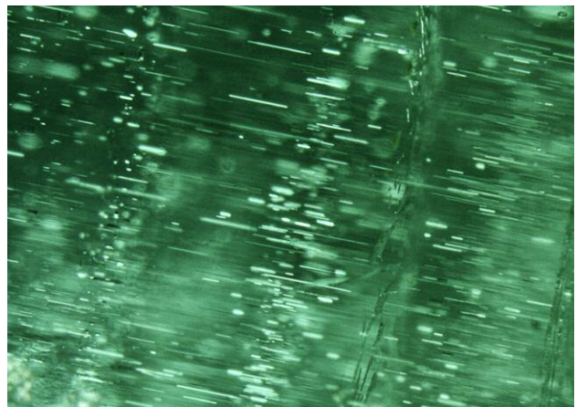
Figure 29. Cloud of fine elongate tubes with various fillings form a rain-like inclusion in a Brazilian emerald. Photomicrograph by Charuwan Khawpong; field of view 1.30 mm.
