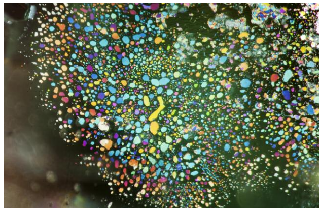
Figure 43. Plane of numerous interference thin films aligned parallel to the basal pinacoid in a Russian emerald. Photomicrograph by Charuwan Khowpong; field of view 1.40 mm.
