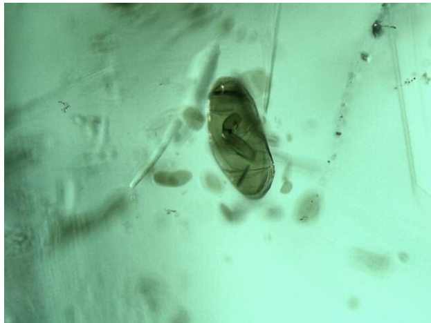
Figure 25. Brownish micas are common in Zambian emerald but can also be found in emerald from other deposits. Photomicrograph by Nattida Ng-Pooresatien; field of view 1.3 mm.
