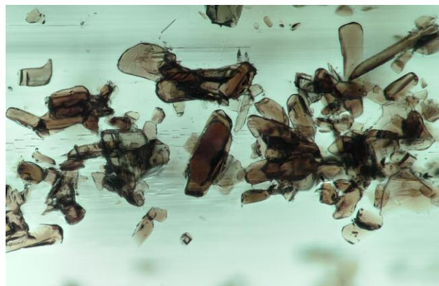
Figure 50. Lath-shaped brown inclusions identified as phlogopite mica in a Russian emerald. Photomicrograph by Suwasan Wongchacree; field of view 1.40 mm.
