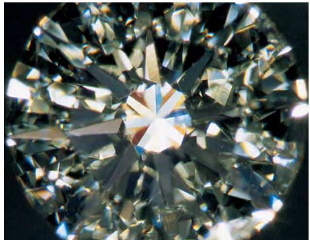
Figure 7. Although synthetic moissanite is typically faceted with the table perpendicular to the c-axis to minimize the effects of double refraction, focusing past the culet will allow doubling to be seen in the reflections of the table and crown facets (left, at 17 \times magnification). This is significantly different from the singly refractive appearance of the facets in diamond (right, at 12 \times magnification). Photomicrographs by Shane F. McClure.
