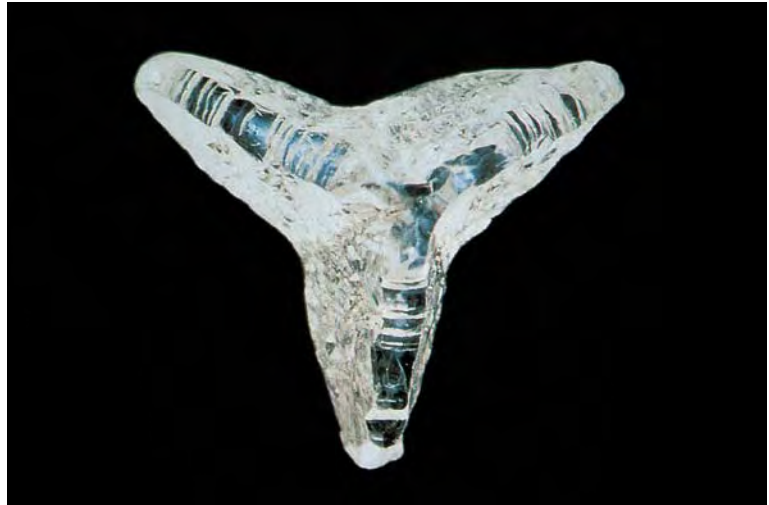
Figure 3. This 0.60 ct slightly etched natural cleavage of a cuboid diamond from the Jwaneng mine, Botswana, shows the “skeletal” appearance that is sometimes formed during cuboid diamond growth. Courtesy of the Diamond Trading Company Research Center, Maidenhead, England; photo by John I. Koivula.
