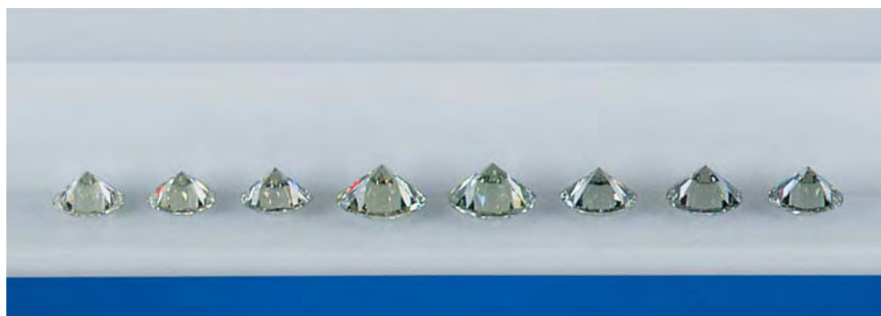
Figure 5. The synthetic moissanites examined at GIA ranged in color from approximately I to U-V on the GIA color-grading scale for diamonds. This range was most evident when the samples were placed table-down and viewed side-by-side in a white plastic tray, as illustrated here. All of the stones had a somewhat gray, green, or yellow appearance. The two largest samples shown here are 1.12 and 1.05 ct. Photo by Shane F. McClure.
