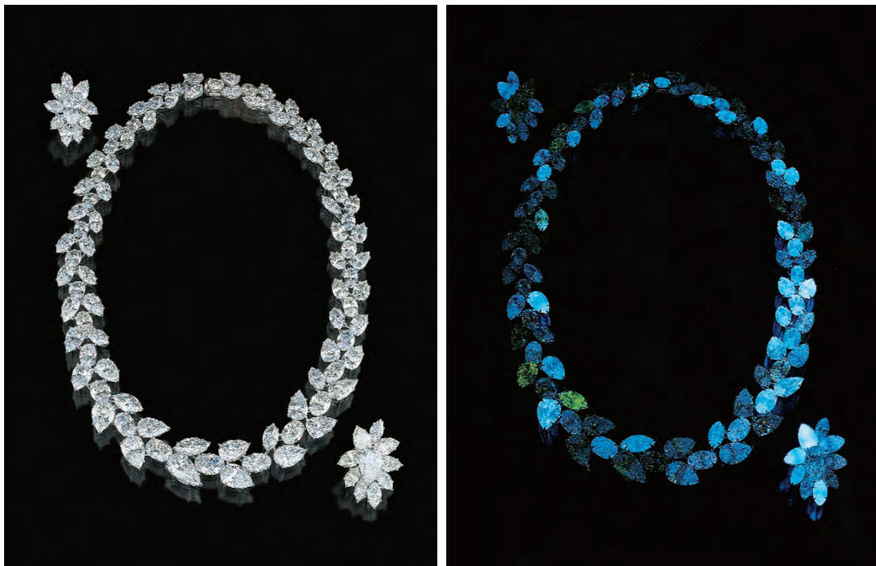
Figure 9. The necklace and earrings reproduced on the cover of this issue of Gems & Gemology are seen here in their entirety under normal lighting conditions (left) and under the long-wave UV lamp (right). Quite often, diamonds in a range of fluorescent strengths and colors are placed next to inert diamonds, yet the piece maintains a uniform overall appearance under normal lighting conditions. The diamonds in the necklace weigh a total of 132 ct; the diamonds in the earrings weigh 23 ct, with the two large pear shapes 3.04 and 3.20 ct. Jewelry courtesy of Harry Winston, Inc.; photos by Harold © Erica Van Pelt.
