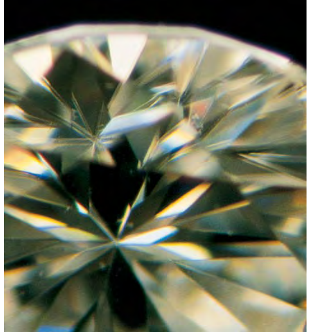
Figure 6. Because of its anisotropic optical character, synthetic moissanite exhibits double refraction depending on the orientation in which a sample is examined. In this view of a faceted synthetic moissanite through the crown main facets, doubling of the facets is readily apparent. Photomicrograph by Shane Elen; magnified 10 \times .
