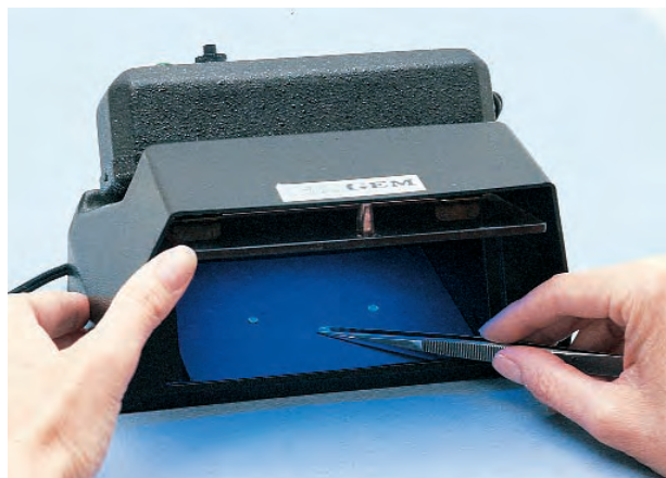
Figure 2. As with diamond color grading, both the control of observation variables (light source, environment, viewing geometry) and the use of known reference stones are required to make consistent fluorescence observations. At GIA GTL, the diamond being examined is placed table-down and moved between the fluorescence reference stones until the intensity of the fluorescence is stronger than the reference stone on the left, and weaker than the reference stone on the right. Photo by Maha DeMaggio.
