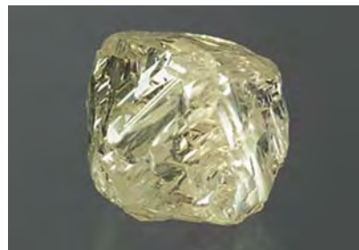
Figure 4. Examination with a desk-model spectroscope proved that this 13.12 ct diamond crystal was treated to enhance its yellow color.
