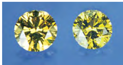
Figure 5. These representative greenish yellow to yellow-green diamonds, each approximately half a carat, were treated by a high-temperature, high-pressure process at GE Superabrasives.
