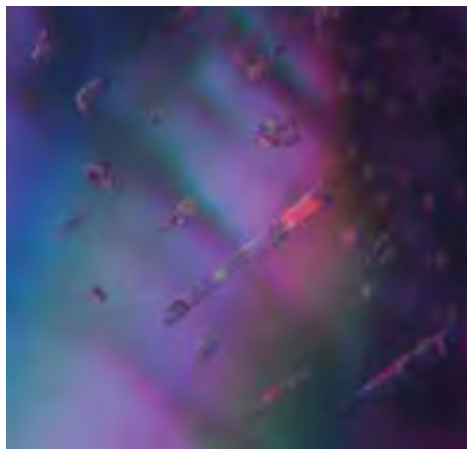
Figure 32. Partially healed fissures in some Winza rubies and sapphires were composed of negative crystals containing multiphase fillings with black-opaque and colorless-transparent (singly and doubly refractive) constituents. Photomicrographs by V. Pardieu/GGL; magnified 60 \times , brightfield (left) and cross-polarized (right) illumination.
