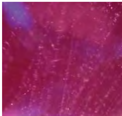
Figure 30. Minute oriented reflective particles were seen in a few samples, generally accompanied by small disk-like inclusions reminiscent of “thin films” (left, magnified 30 \times ). Less common are coarser particles present in diffuse clouds or stringer-like formations (right, magnified 80 \times ). Photomicrographs by V. Pardieu/GGL; fiber-optic illumination.
