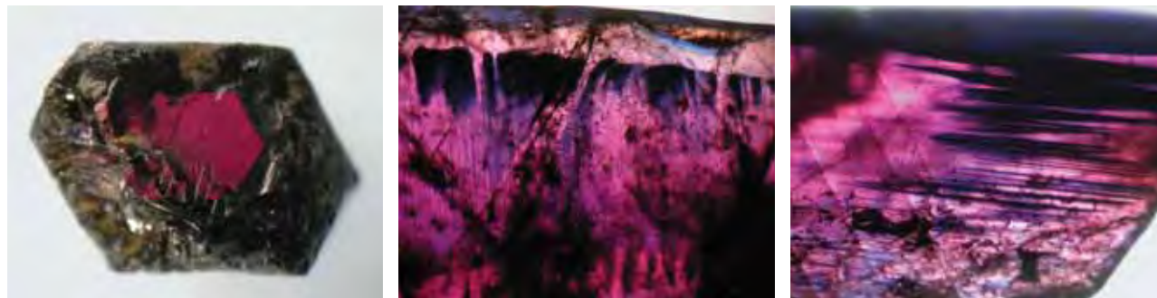
Figure 21. Viewed parallel to the c -axis, the 7-mm-wide dipyramidal corundum crystal on the left has a ruby core and a dark violetish blue (nearly black) rim. When another dipyramidal sample (center) is viewed perpendicular to the c -axis (which is horizontal in this photo), the bluish violet areas are restricted to small zones close to the rim. The rhombohedral sample on the right, which is also seen perpendicular to the c -axis (vertical in this photo), has bluish violet zones that appear as thin layers parallel to the basal pinacoid c . Photomicrographs by K. Schmetzer; center and right taken in immersion, magnified 50 \times .
